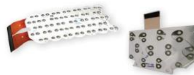
Monitoring bus bar examples for battery connections
